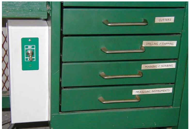
DC Drive Box tucked away under the bench. (note the Spindle Reverse Switch mounted on the box) {Shown without safety-flap}
