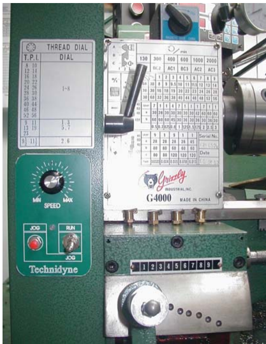
Lathe-Mounted Control Panel
