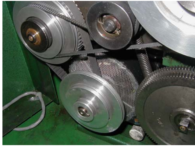
The pulley arrangement (note filter)
