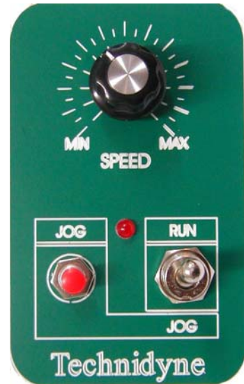
Close-up of Control Panel (made on my CNC Engraver/Router)
