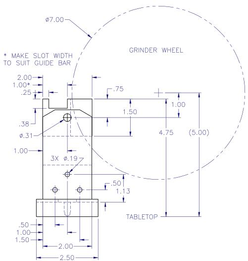
TOOL GRINDING REST ASSY & DETAILS
